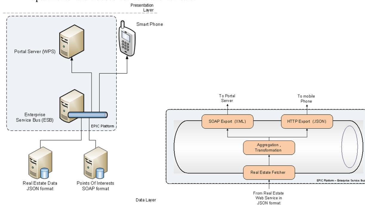
Figure 4: Architecture and Information Flow of the Relocation Application
